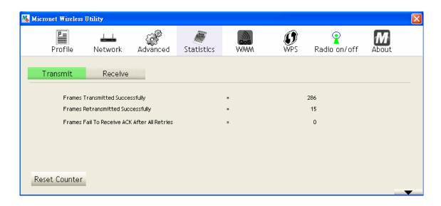
All connection-related statistics is displayed here. Users can click 'Transmit' or 'Receive' tab, to view the statistics of transmitted or received packets. It can also click 'Reset Counter' button, to reset the statistics of all items back to 0.
